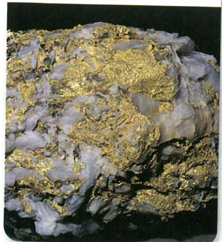
■ Figure 6.21 When the hydrothermal solution in the quartz cooled, gold veins formed.
